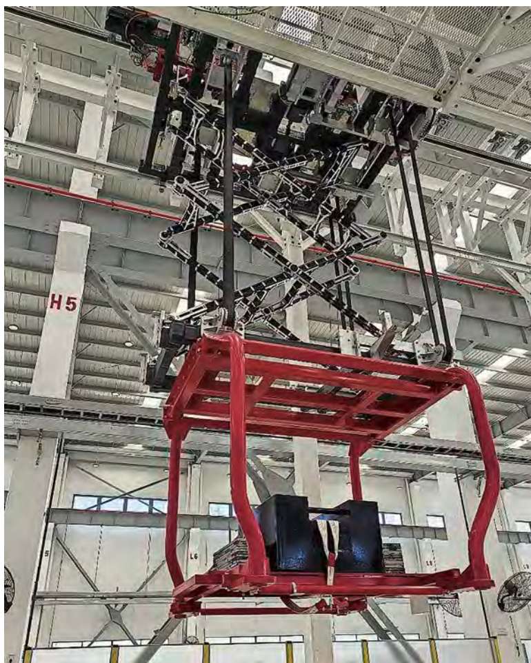
Electric monorail system with scissor lift extended
