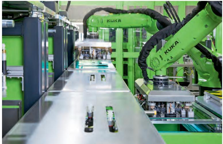
ner points of the ready-cut tape are determined and the results are referenced against the tool centre point of the EOAT.
