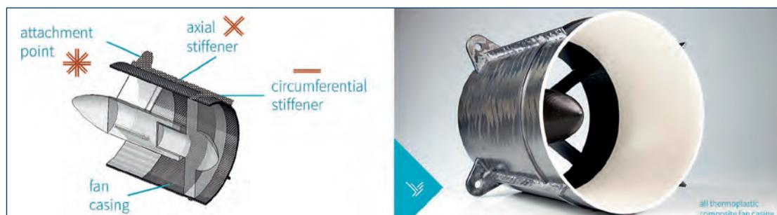
Part design with fiber orientation of the functional elements; demonstrator
