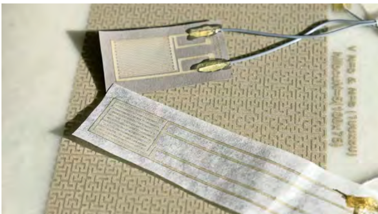
Paper-based cure monitoring, strain, moisture, and crack detection sensors
