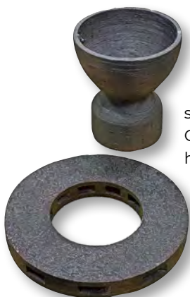
Examples of 3D-printed CMCs
