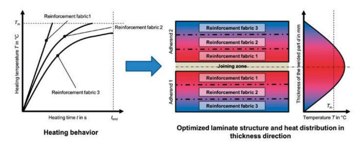
Fig. 1: Optimization of the laminate structure regarding higher welding speeds after heating-up tests of several reinforcement fabrics
