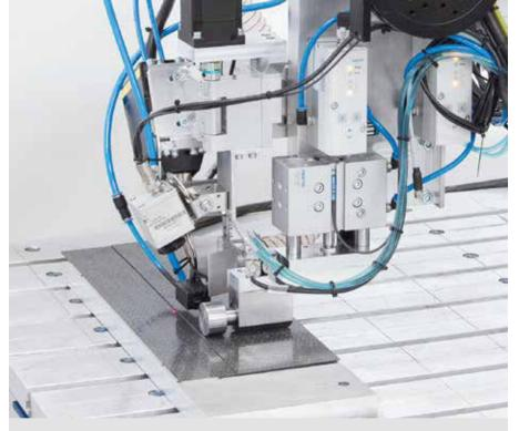
*Fig. 2: Induction welding head for continuous induction welding of CFRPC (developed by Pfaff Industriesysteme und Maschinen).*
