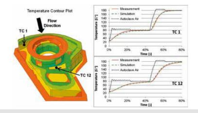
*Fig. 2: H145 Fenestron™ shroud tooling thermal simulation: Comparison of the thermal simulation developed by Airbus Helicopters Deutschland GmbH with experimental measurement of the temperature distribution on the mold surface during a standard autoclave cycle.*
