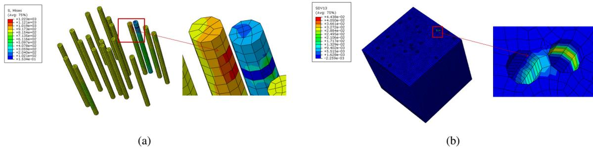
**Figure 4.** (a) Local load sharing after first fiber break. (b) Matrix plasticity after first fiber break.
