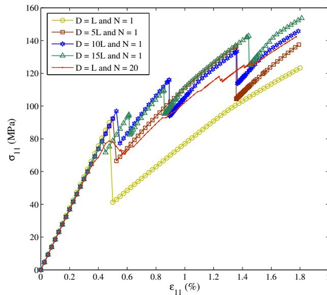
**Figure 2.** Homogenized stress strain curves for  $D = L, 5L, 10L$  ( $N = 1$ ) and  $D = L$  ( $N = 20$ ) with varying strength along the fiber.
