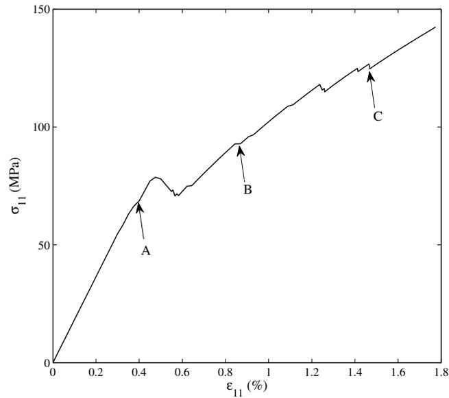
**Figure 3.** Homogenized stress strain curves for  $D = L$  ( $N = 20$ ) with varying strength along the fiber.
