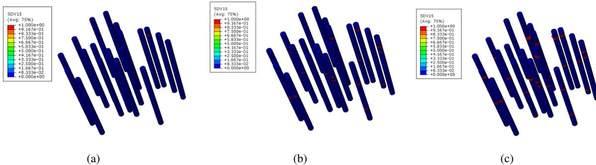
**Figure 5.** (a) Failed elements in fiber corresponding to point A (b) Failed elements in fiber corresponding to point B (c) Failed elements in fiber corresponding to point C
