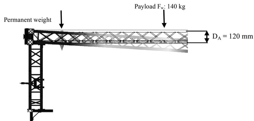
**Figure 5.** FEM Analyses of cabin arms (bending scaled 10:1).
