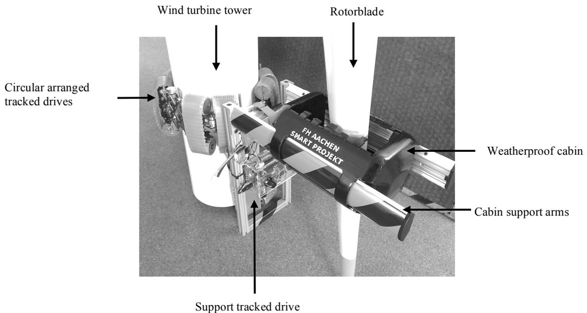
**Figure 2.** SMART Modell (scaled 1:20).
