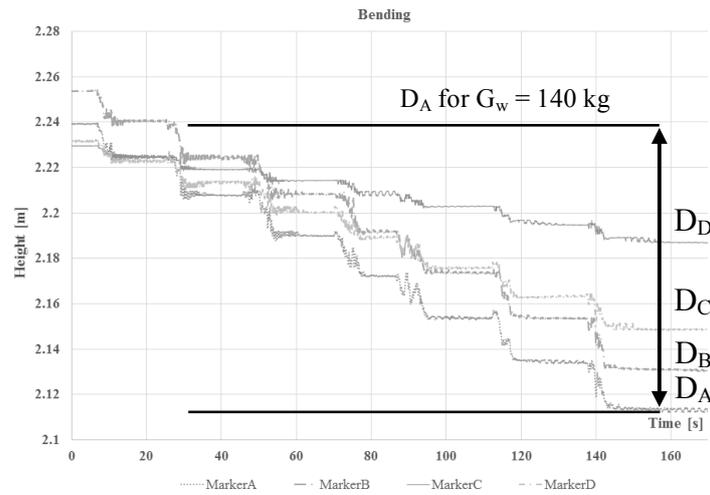
**Figure 4.** Initial bending of the cabin arms.
