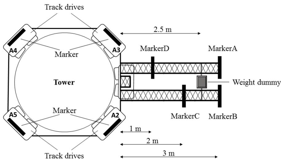
Figure 3. Marker and weight dummy attached to extension arm.
