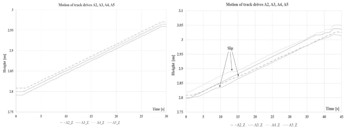
**Figure 6.** Test drive without load (left) and a weight dummy (right).
