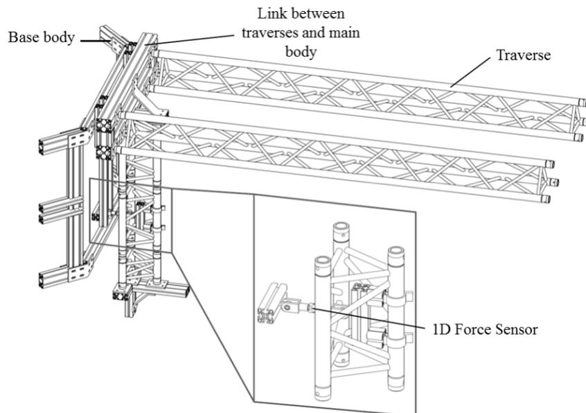
**Figure 8.** Load sensor for cabin.
