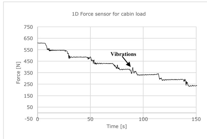
**Figure 9.** Measurements of the initial load with force sensor.
