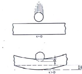
**Figure 1.** Local and overall deformation of flexible target [10]
