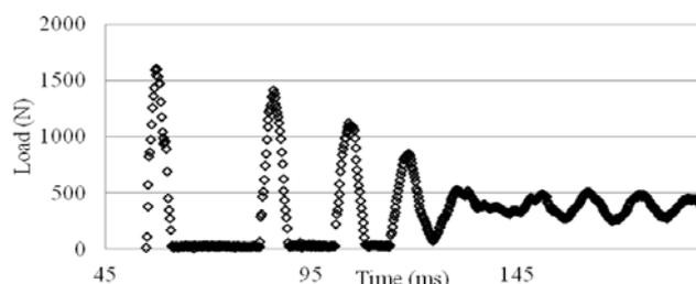
**Figure 5.** Load versus time for an 11 J (4.5 bar) impact with a semispherical indenter
