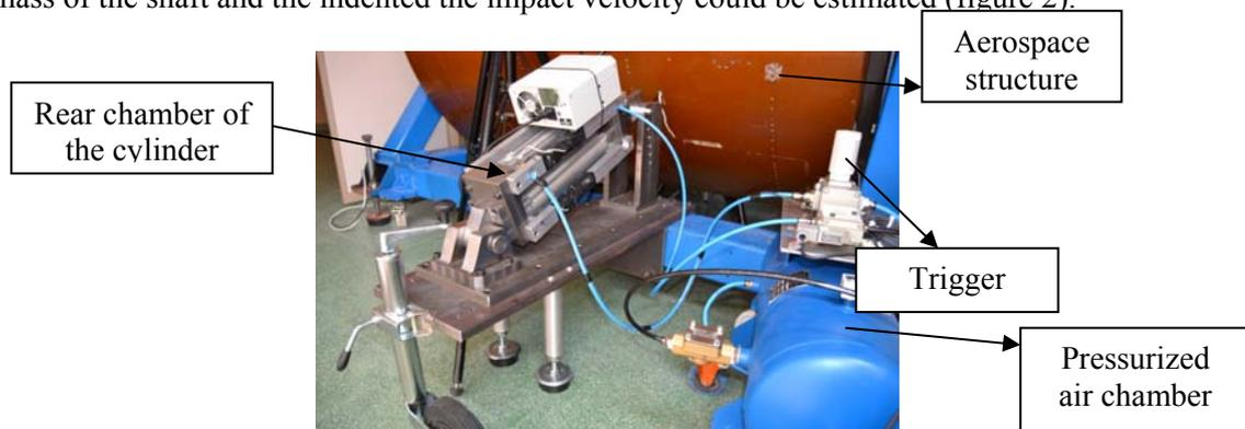
**Figure 2.** Impact device developed for experiments on a real aerospace demonstrator
