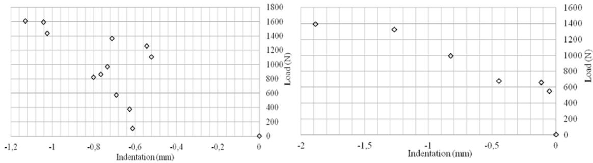
**Figure 8.** Contact law for an impact test using a semispherical indenter. A) 11 J. B) 18 J
