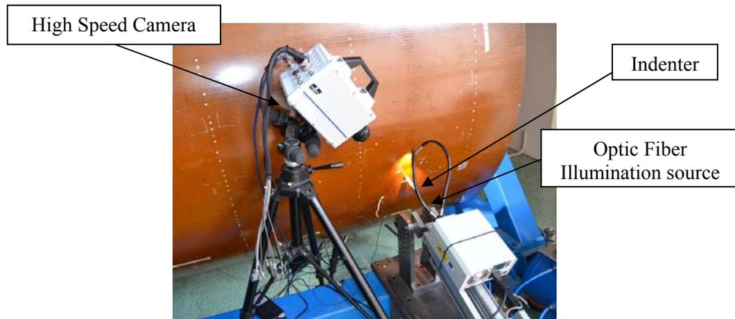
**Figure 3.** Adopted experimental set up placed at the front face of the aerospace panel
