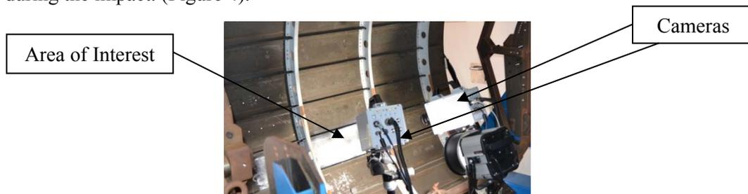
**Figure 4.** Adopted experimental set up placed at the rear face of the aerospace panel
