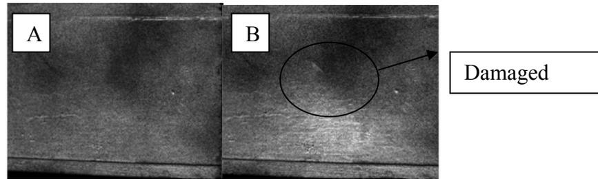
**Figure 6.** A) Reference image previous to the impact for a 11J experiment). B) Image during the impact for an 11J experiment.
