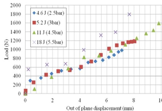
**Figure 7.** Out of plane displacements versus load during the different impact test performed using a semispherical indenter.
