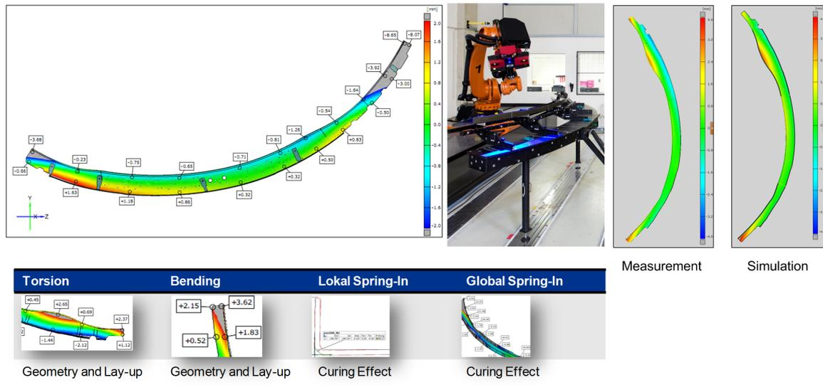
**Figure 6.** Measured distortions and deformation modes of composite frames (left), comparison of simulated and measured distortions (right)
