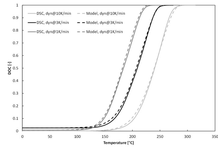
**Figure 2.** Experimental DSC data and cure kinetics model predictions: dynamic (constant ramp rate).
