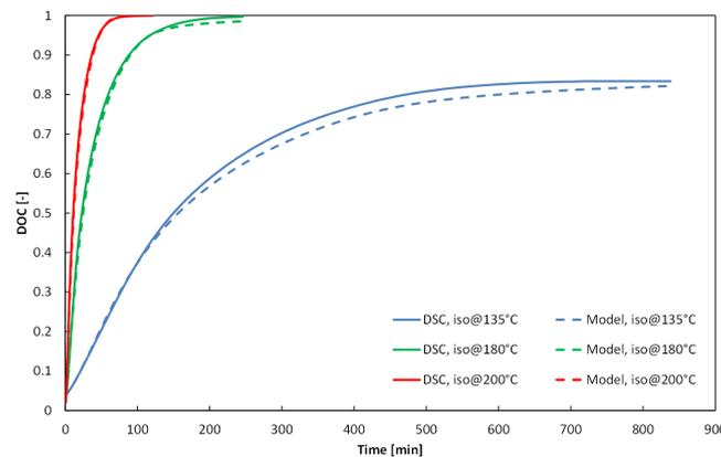
**Figure 1.** Experimental DSC data and cure kinetics model predictions: isothermal.
