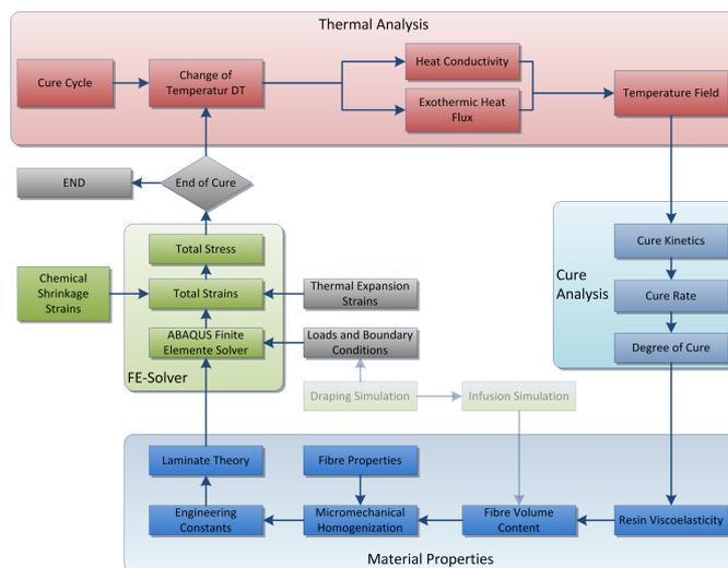
**Figure 5.** Finite element simulation work flow for the determination of curing induced distortions.
