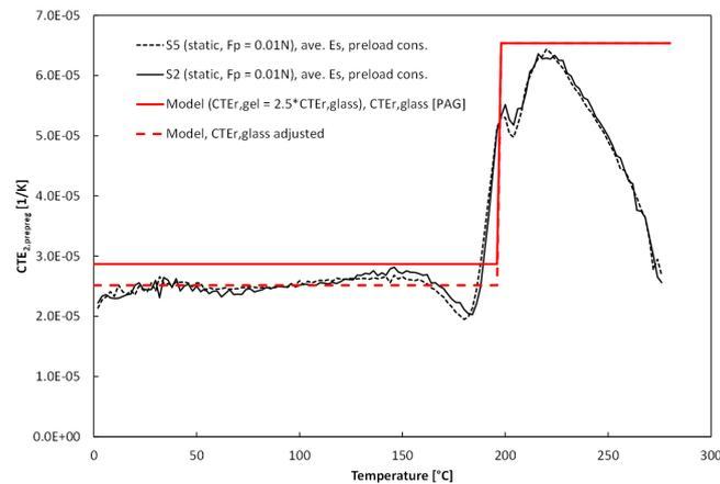
**Figure 4.** Variation in composite fibre transverse CTE from DMA tests and model fit.
