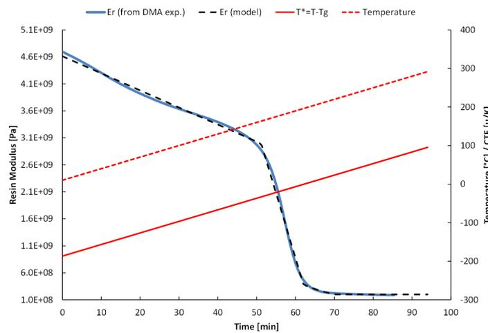
**Figure 3.** Resin modulus progression from DMA tests and model fit.
