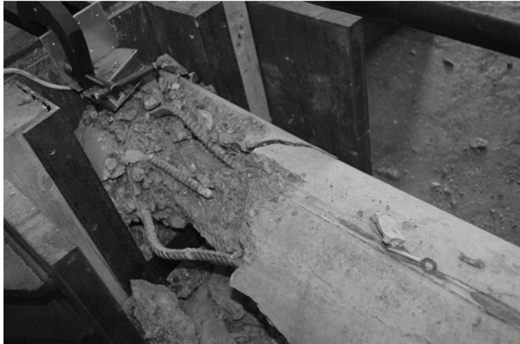
**Figure 3.** Failure mode of the column C-2 with steel reinforcement.
