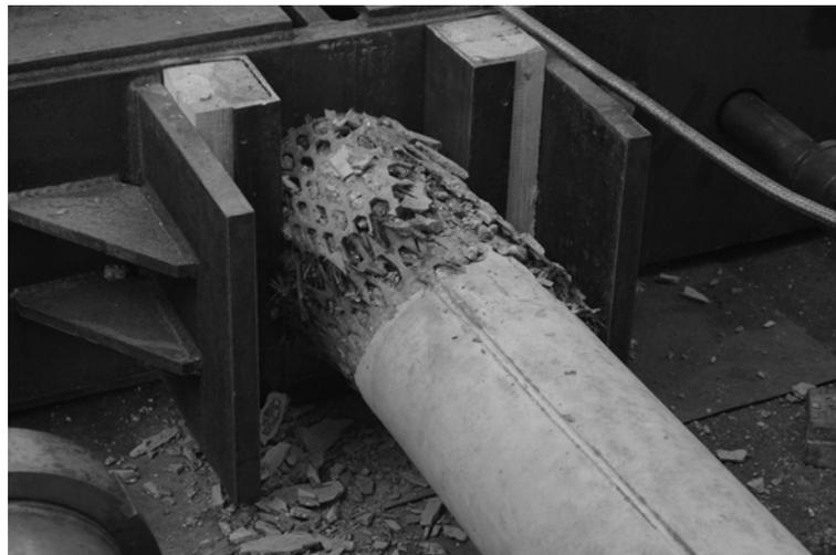
**Figure 4.** Failure mode of the column C-3 with anisogrid lattice composite reinforcement.
