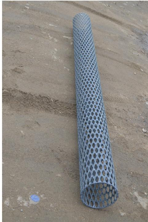
**Figure 2.** Anisogrid lattice composite reinforcement of C-3 Column.
