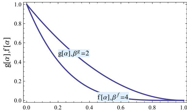
**Figure 2.** Damage degrading functions  $f[\alpha]$  and  $g[\alpha]$ .
