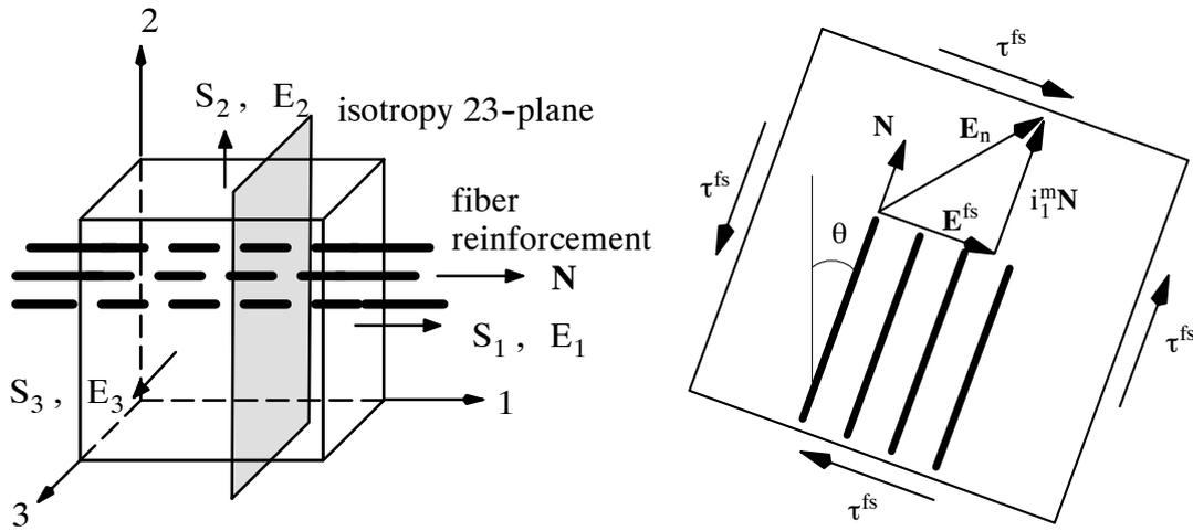
**Figure 1.** a) A UD laminate in transverse isotropy with fibre orientation  $N$ . b) Fibre/matrix shear stress  $\tau^f$  associated with fibre/matrix shear strain  $\gamma^f$ .
