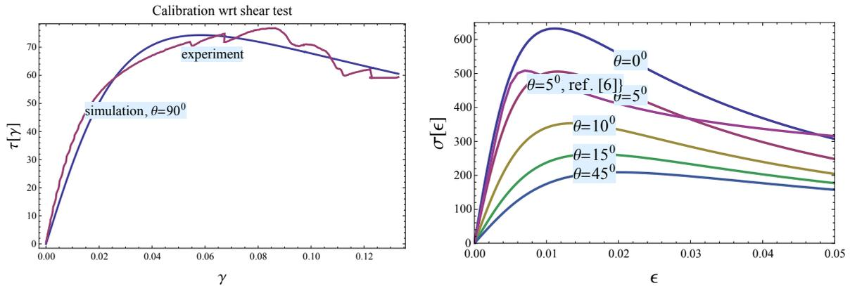
**Figure 3.** a) Model calibration result with respect to an in-plane pure shear test performed on a unidirectional laminate. b) Uniaxial compressive response for different fibre kinking of the present model compared to a kinking model developed in [6].
