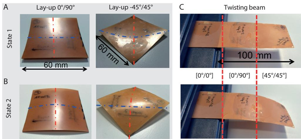
**Figure 2.** A-B) Platelet-reinforced bi-stable square plates: A) bending and B) twisting specimens with  $[0^\circ/90^\circ]$  and  $[-45^\circ/45^\circ]$  lay-ups, respectively. C) Juxtaposition of three lay ups featuring different micro-reinforcement architectures:  $[0^\circ/0^\circ]$ ,  $[0^\circ/90^\circ]$  and  $[-45^\circ/45^\circ]$  producing a bending-twisting multi-stable beam.
