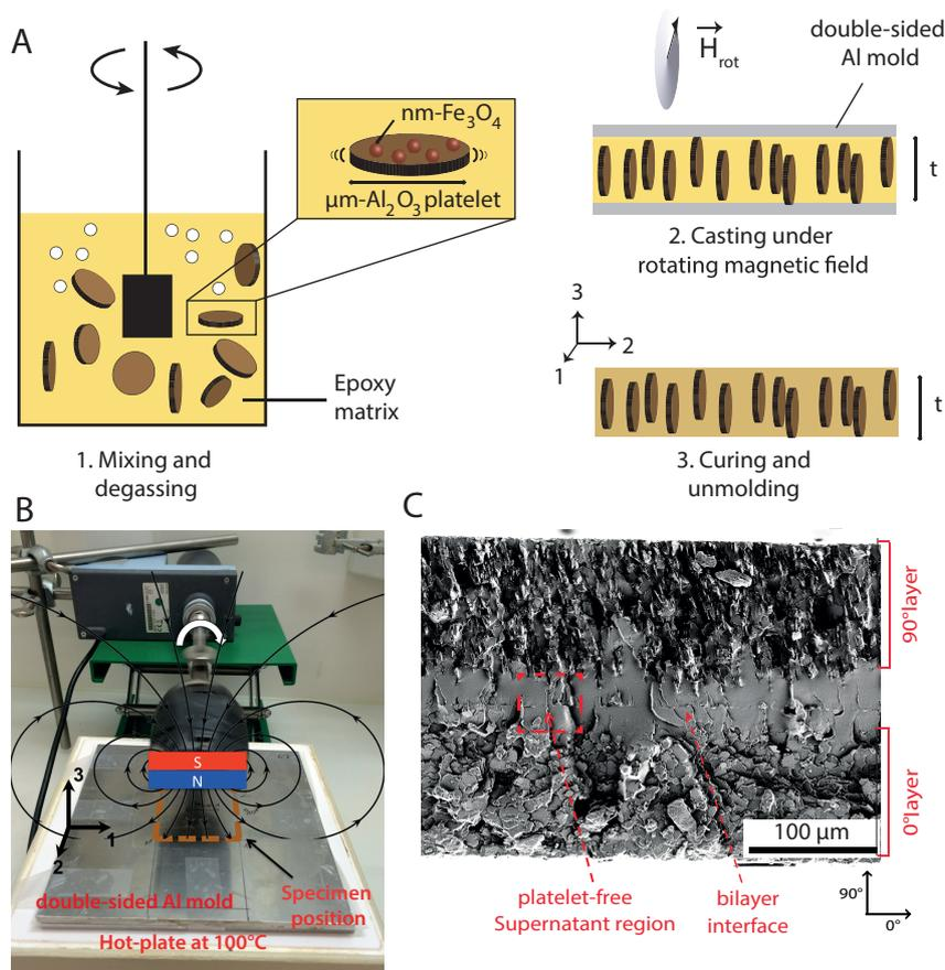
**Figure 1.** Procedure for the fabrication of anisotropic single layers with controlled thickness using the set-up shown in B). The magnetic field is rotated within the plane parallel to vectors 1 and 3. C) SEM micrograph of a cross-section of a  $[0^\circ/90^\circ]$  lay-up bilayer.
