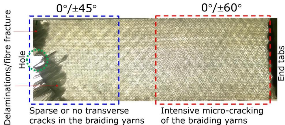
**Figure 3.** Fractured steered braided composite in transmitted light showing variation in transverse matrix cracking over the sample length and failure zone
