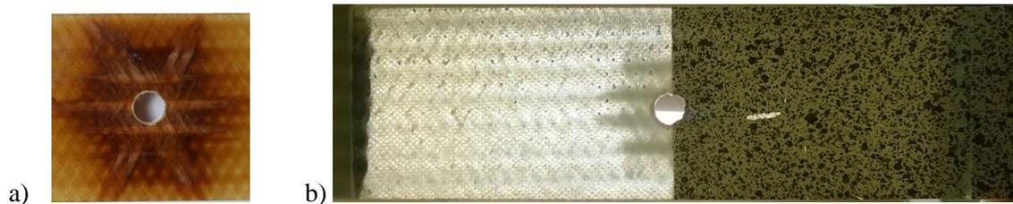
**Figure 1.** a) CE patch in the sample with hole (the hole diameter is 6 mm), b) The sample patched with core-shell rubber toughened epoxy (the right side of the samples shows DIC speckling).
