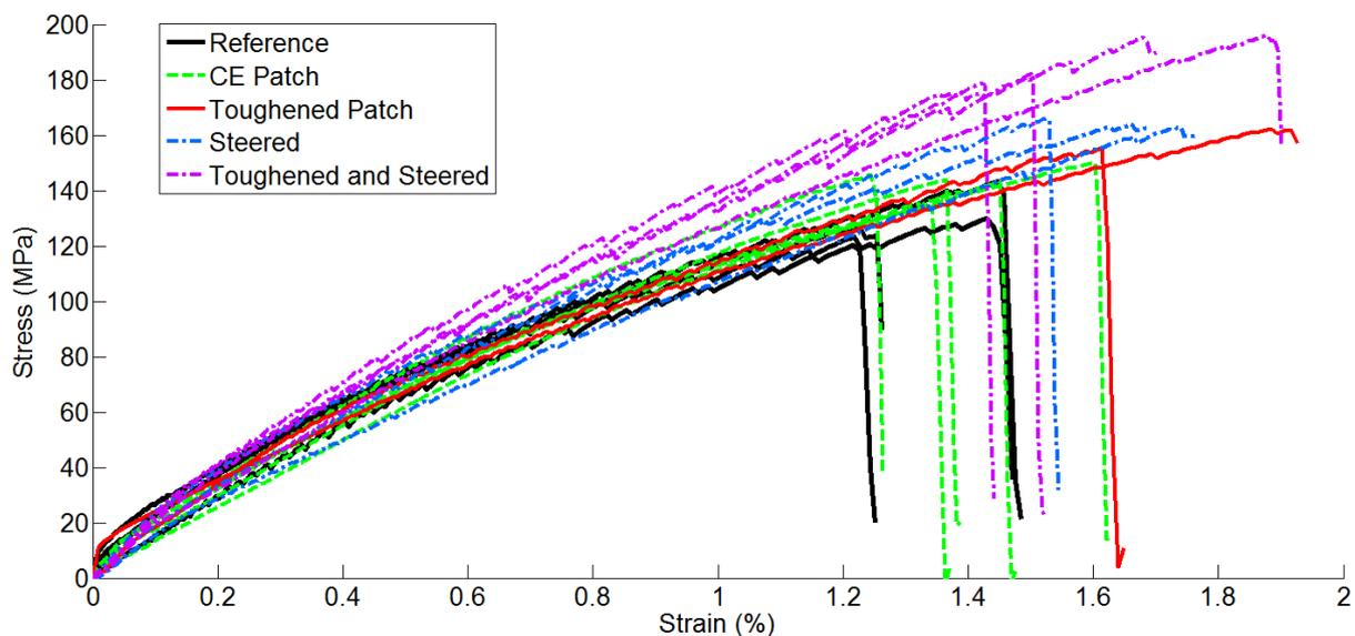
**Figure 2.** Stress-strain diagrams for all the samples discussed in the study.
