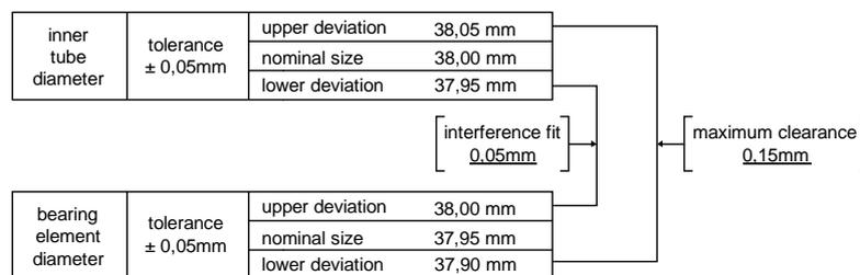
Figure 6. Selection of the tolerance field for the tube and the bearing
