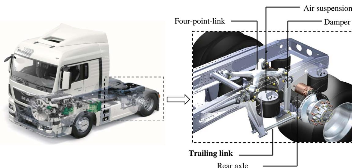
Figure 1. MAN TGX long-haul transport vehicle – component illustration of the rear axle
