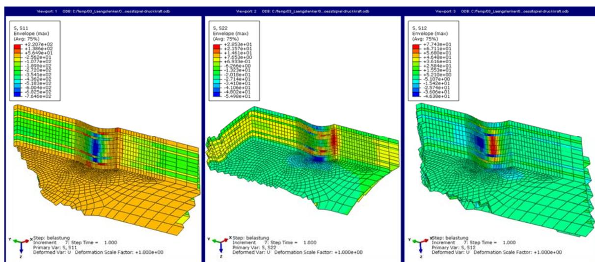
**Figure 7. Stress components S11 (longitudinal stress), S22 (transverse stress) and S12 (shear stress) in the area at the end of the slot (load case 1: maximum compression load; tolerance field: interference fit)**
