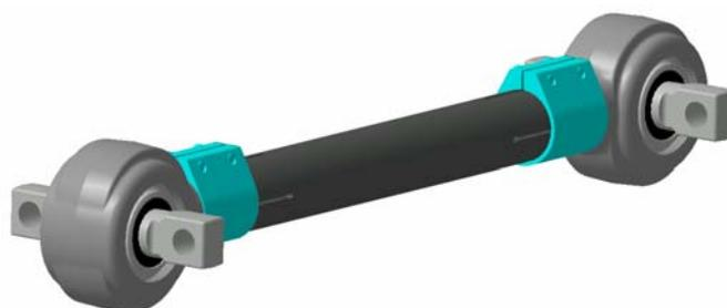
**Figure 8. Final concept of the trailing link**
