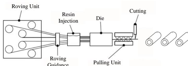
Figure 4. Pultrusion process for continuous manufacturing of profiles [3]
