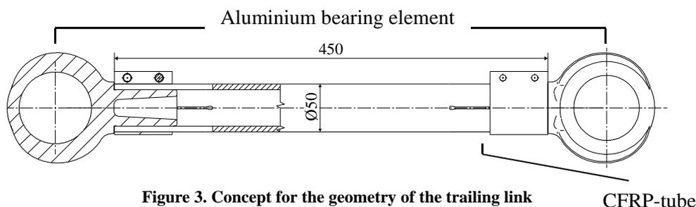
Figure 3. Concept for the geometry of the trailing link
