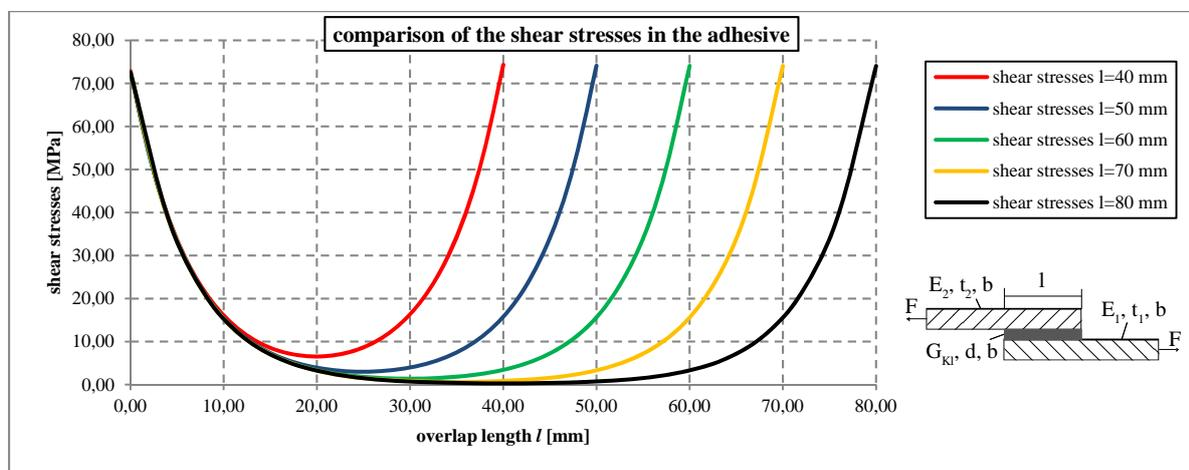
**Figure 5: Shear stresses in the adhesive for various overlaps  $l$**
