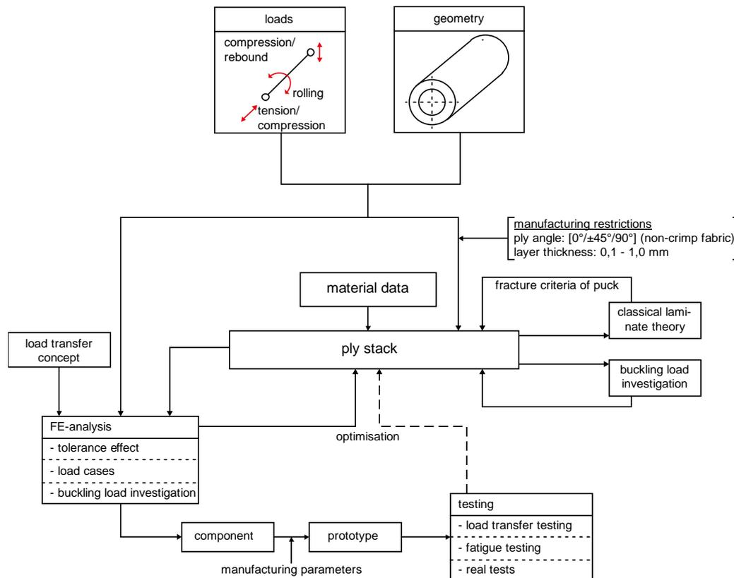
Figure 2. Development steps of the trailing link
