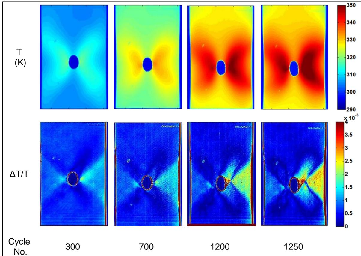
**Figure 4.** (+/-45) Specimen temperature evolution.
