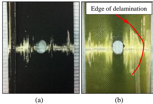
**Figure 3.** Photo of the failed (0, 90) Specimen, after 140,922 cycles (a) front face (b) back face.
