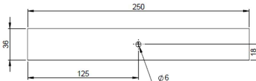
**Figure 1.** Dimensioned drawing of the composite open hole specimen.
