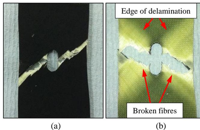
**Figure 5.** (+/-45) Specimen failure image after 1291 cycles. (a) front face (b) back face.
