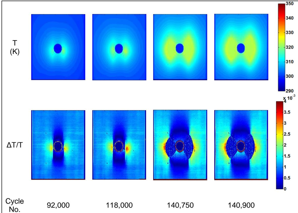
**Figure 2.** (0, 90) Specimen temperature evolution.
