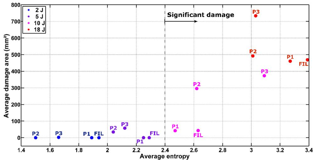
**Figure 6.** Average damage areas vs initial transients average entropies ( $N = 103$ )
