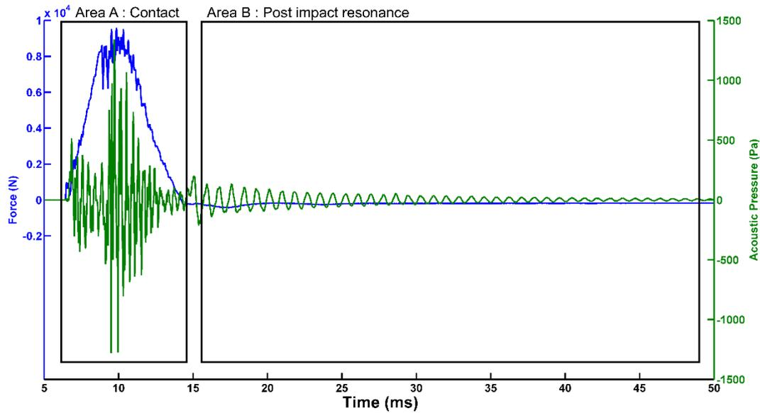
**Figure 2.** Force and acoustic signal for an 18 J impact test on FIL stacking sequence.
