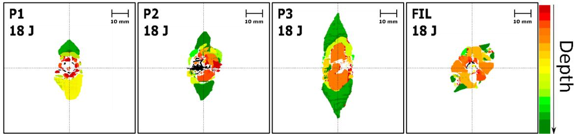
**Figure 4.** Post mortem ultrasonic scans: damaged areas for 18 J impacts on each stacking sequence.
