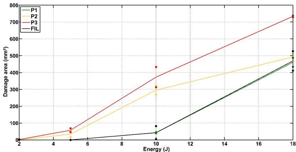
**Figure 5.** Average damage areas for all stacking sequences
