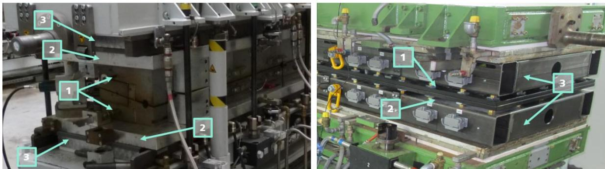
**Figure 1.** Aluminium tool used for Prepreg technology (1-cavity, 2-heat-/and cooling plate, 3-transportation device) (left); CFRP tool used for RTM technology (1-upper mould, 2-lower mould, 3-steel frame) (right)
