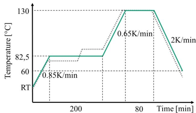
**Figure 4.** Adapted Prepreg cycle for the aluminium tool
