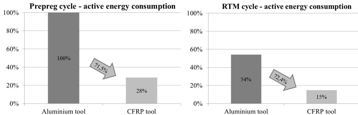
**Figure 5.** Calculated energy demand of the aluminium tool and the CFRP tool referred to the adapted Prepreg cycle (left) and referred to the RTM cycle (right).
