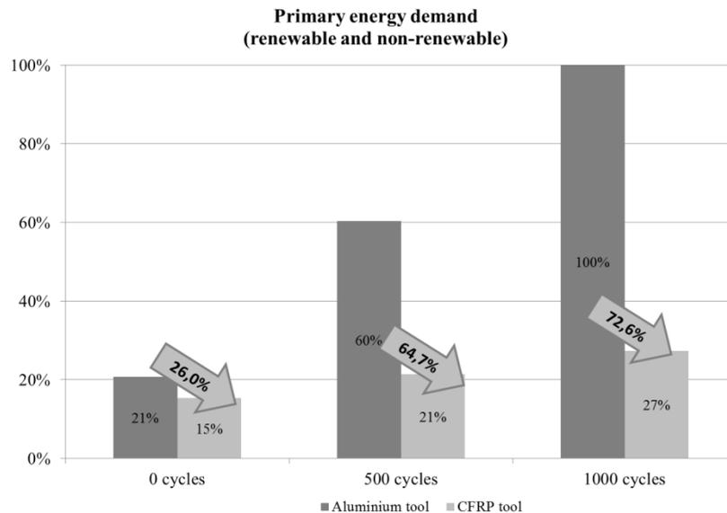
**Figure 6.** Primary Energy Demand (PED) for the manufacturing of the aluminium tool in comparison to the CFRP tool and with the consideration of 500 and 1000 use-phase cycles.
