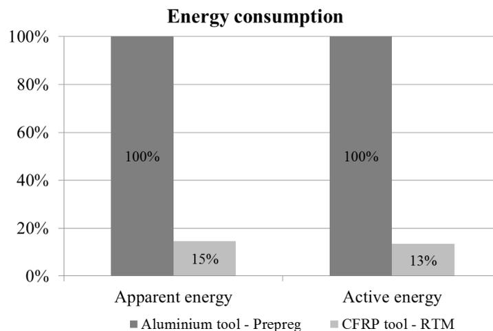
**Figure 3.** Relative energy consumption of the aluminium and the CFRP tool in comparison for one complete curing cycle.
