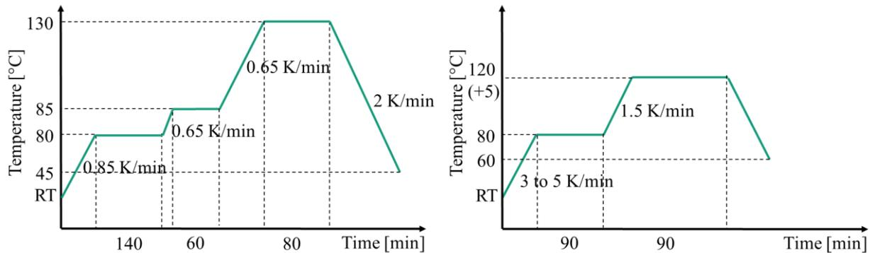
**Figure 2.** Prepreg curing cycle for the amluminium tool (left) and RTM curing cycle for the CFRP tool (right)
