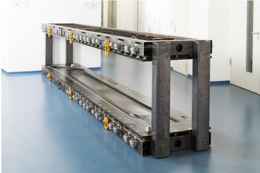
**Figure 7.** CFRP RTM tool with integrated heating, developed and manufactured by QPoint Composites GmbH for manufacturing a full size helicopter rotor blade with an approx. length of 5 meters, exhibit at the project partner (LCC Technische Universität München) site.
