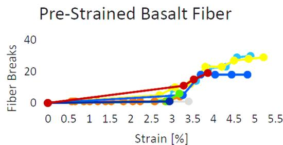
**Figure 5:** Fiber breaks vs. strain in basalt fiber
