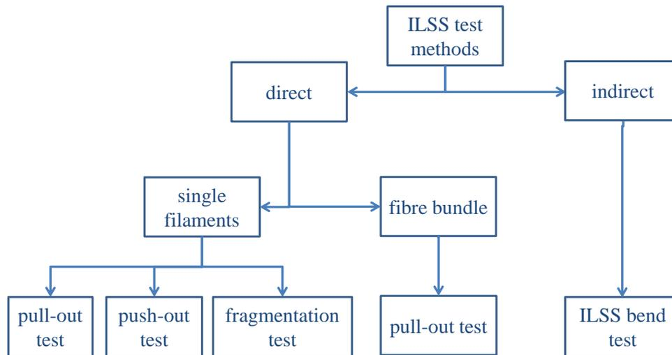
**Figure 1:** Overview about different test methods for the interlaminar shear strength (ILSS)
