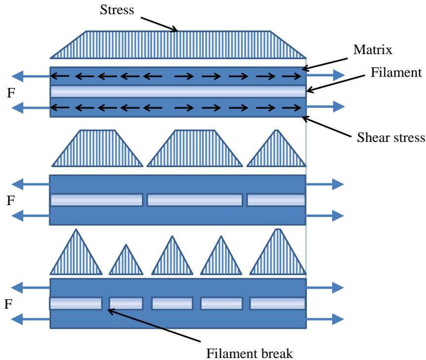
**Figure 3:** Tension distribution during the single filament fragmentation test [5]
