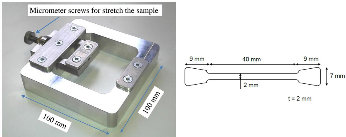
**Figure 4:** Tenter (left) and sample geometry (right)
