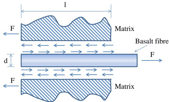
**Figure 2:** Interlaminar shear stress (ILSS) between fiber and matrix. [5]
