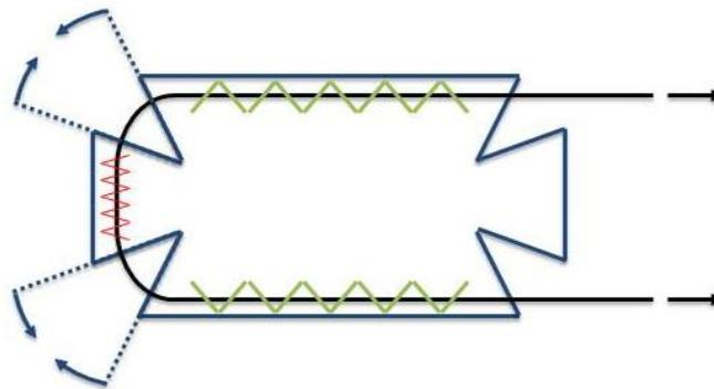
**figure 8:** Closing base material cuts by selective tow manipulation using different TFP stitching parameters.
