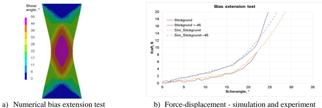
**figure 3:** Bias Extension test for base material.
