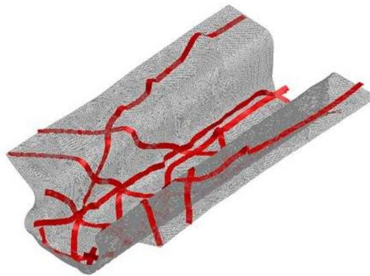
**figure 5:** Reverse draping simulation of base material and reinforcing yarns.
