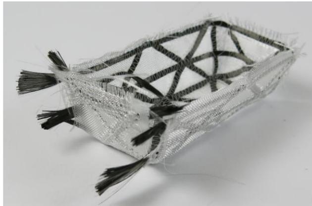
**figure 10:** Three-dimensional preform resulting from the forming process using selective fibre manipulation.
