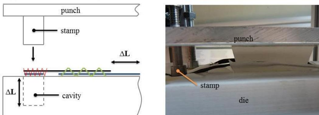
**figure 9:** Selective tow manipulation. Left: schematic illustration, right: real application.
