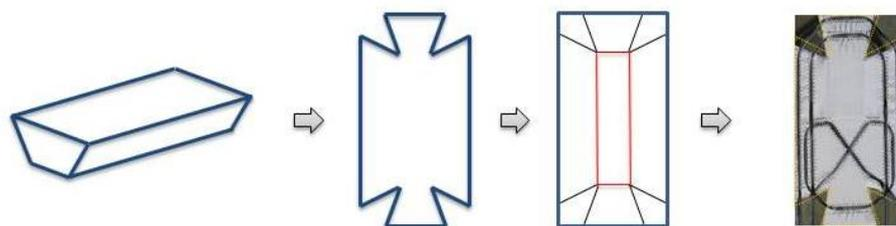
**figure 7:** Deduction of the base material geometry. From left to right: part geometry, unfolded contour plot, plot with folding and cutting lines, realisation of base material.
