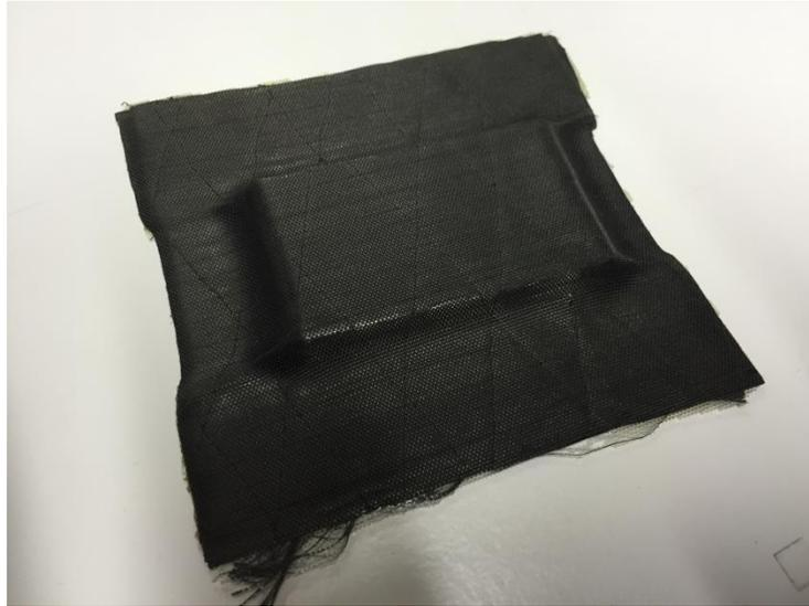
**Figure 2.** 3D composite cured with accelerator.
