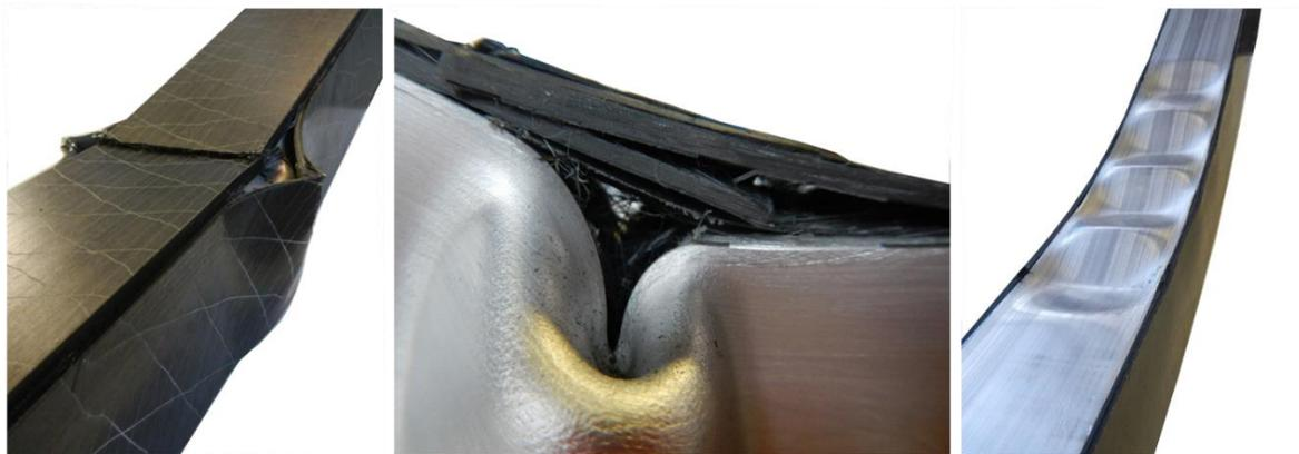
**Figure 3.** Typical failure mechanisms. (left) introduced web buckling after compressive instability fiber cracking at flange. (middle) cfrp fiber cracking (SHS7). (right) plastic flange buckling (SHS5)
