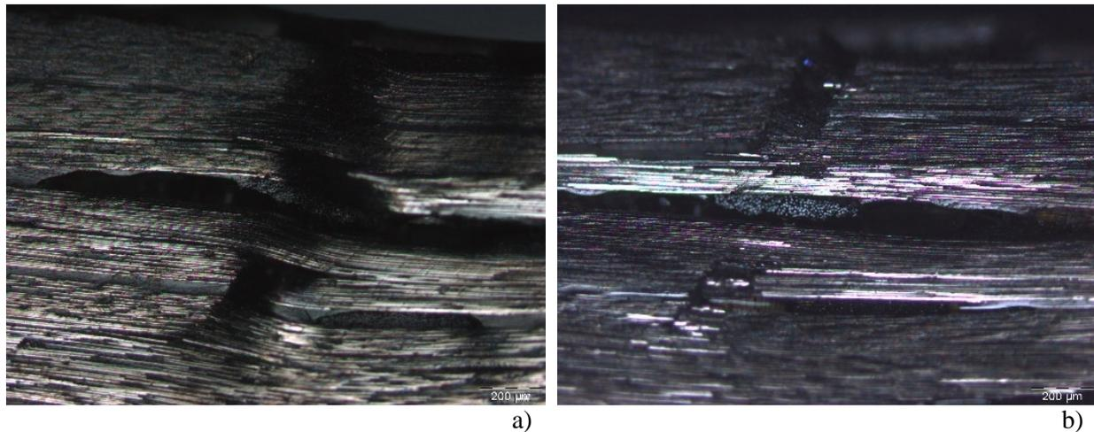
**Figure 6.** Optical micrographs on a delaminated sample with fibre breakage.
