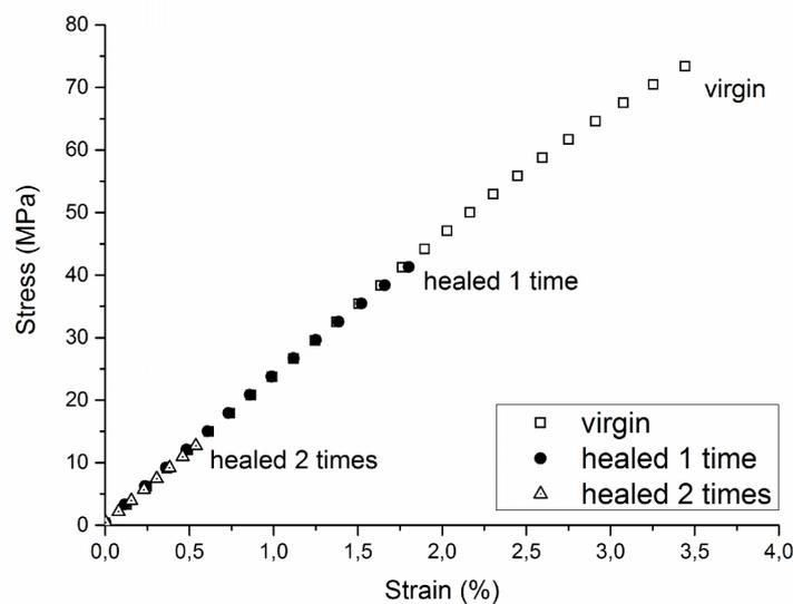
**Figure 3.** Three point bending on as prepared and healed samples
