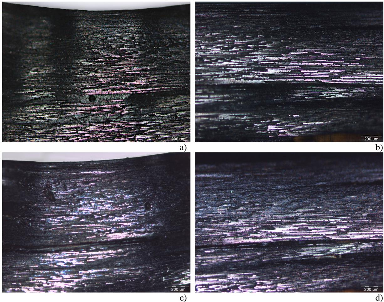
**Figure 4.** Optical micrographs on a delaminated sample.
