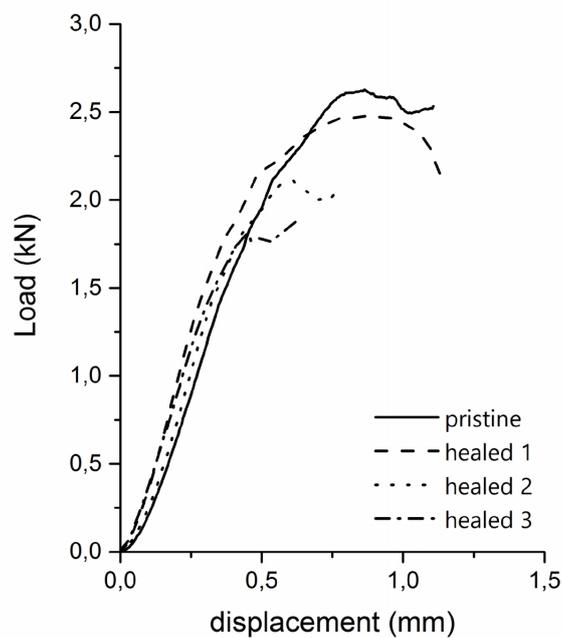
**Figure 5.** Short Beam test on composite sample
