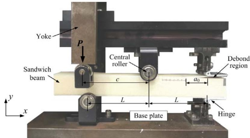
**Figure 1.** Sandwich beam specimen with initial debond loaded in the MMB test rig
