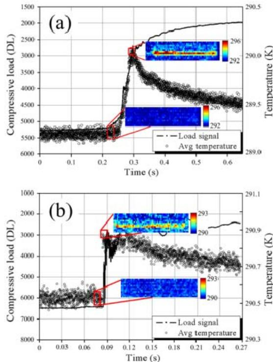
**Figure 3.** Load and average temperature trace obtained from specimens with (a) crack propagation path in the core, and (b) crack propagation path at the face/core interface
