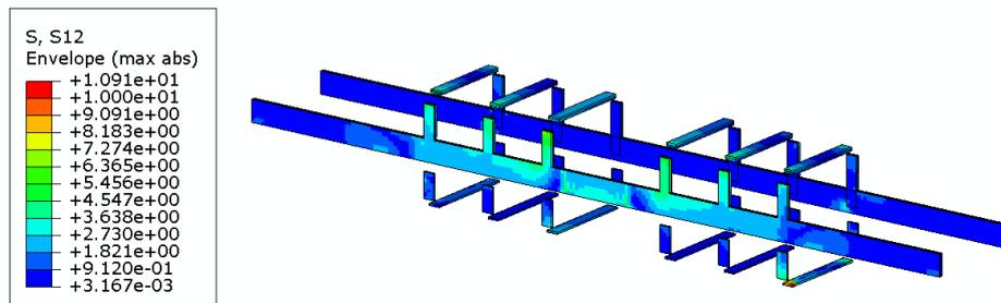
**Figure 6.** Shear stress in the adhesive interfaces.
