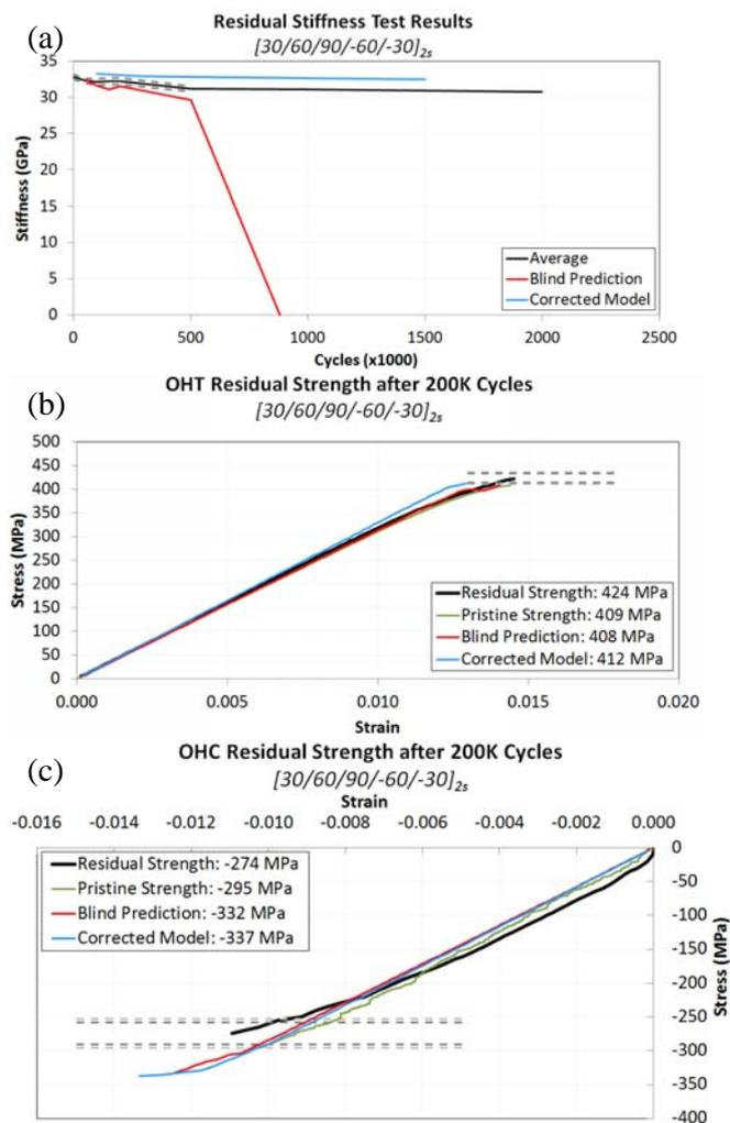
**Figure 4.** (a) Residual stiffness, (b) OHT residual strength, and (c) OHC residual strength predictions and experiments for the  $[30/60/90/-60/-30]_{2s}$  laminate at 200k cycles.
