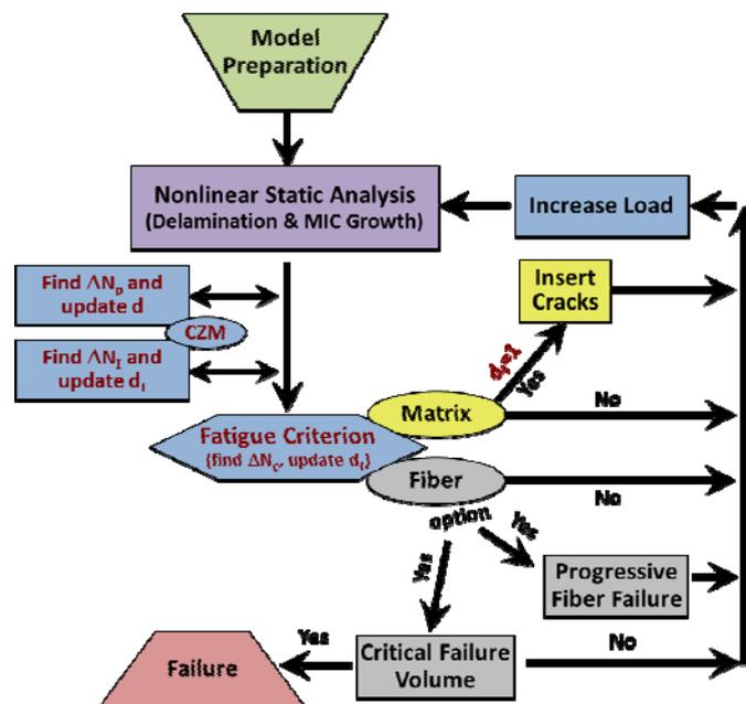
Figure 2. Fatigue DDM Algorithm
