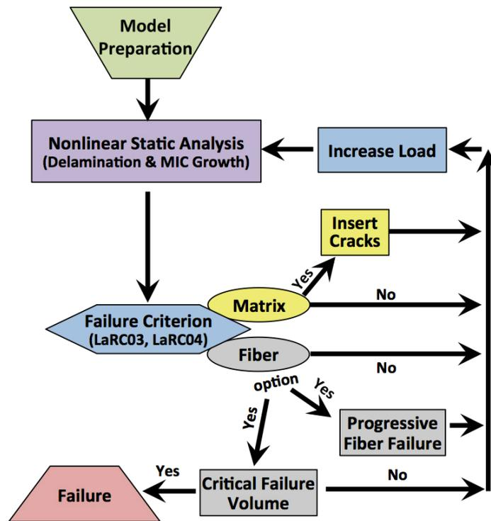
Figure 1. Static Solution Algorithm
