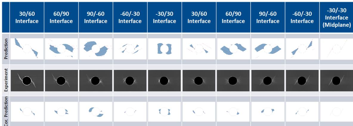
**Figure 3.** Delamination extent in  $[30/60/90/-60/-30]_{2s}$  laminate after 200,000 cycles.
