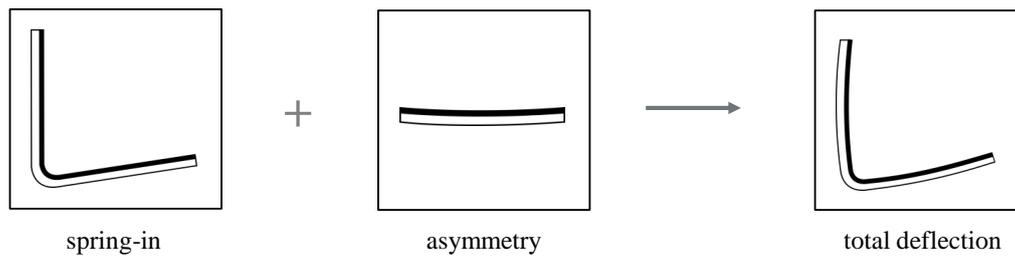
**Figure 4:** The total deflection of RTM-parts is driven by two main underlying mechanisms: spring-in and asymmetry. As representation for possible asymmetries and  $V_f$ -gradients in thickness-direction, neat resin layers on L-shaped CFRP-specimens are investigated.
