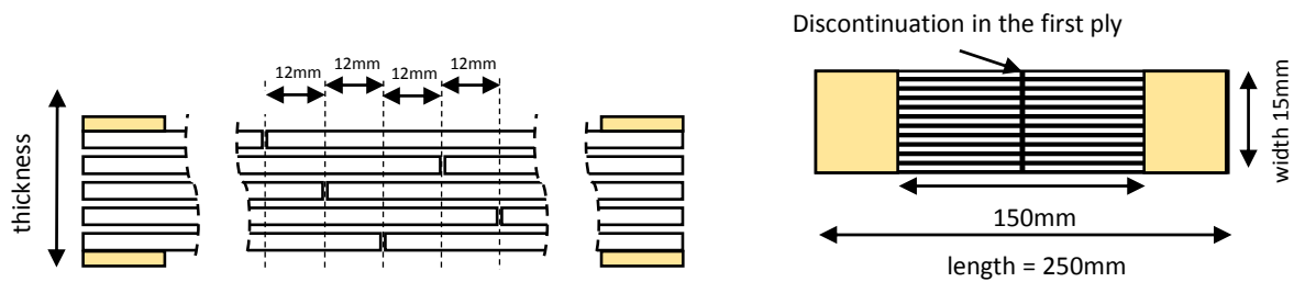
Figure 2. Patch pattern (left) and specimen dimensions (right)
