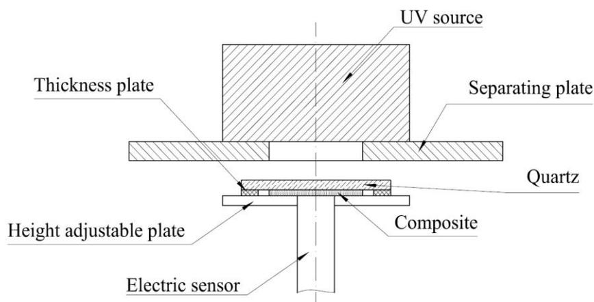
**Figure 2.** Description of the curing analysis system
