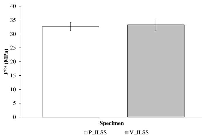
**Figure 5.** Short-beam strength for manufactured specimens.
