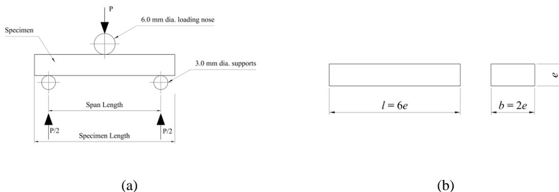
**Figure 3.** (a) Horizontal shear load diagram. (b) ILSS specimen configuration.
