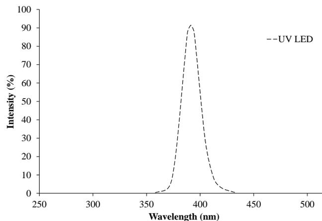
Figure 1. Emission spectrum of the UV LED.
