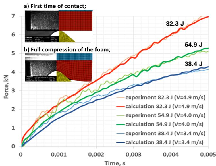
**Figure 6.** Validation result with kerbstone (Foam density = 60 g/L, high temperature ( $\approx 50^{\circ}\text{C}$ )).
