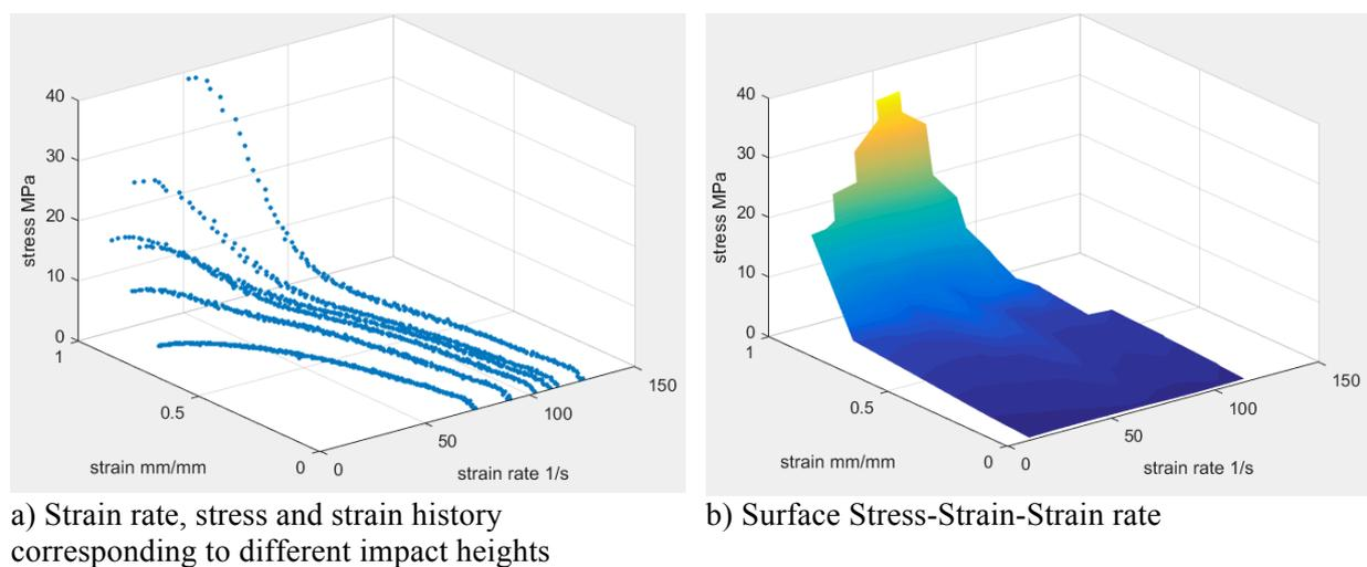
**Figure 3.** Experimental results (Foam density = 80 g/L, room temperature ( $\approx 18^{\circ}\text{C}$ )).
