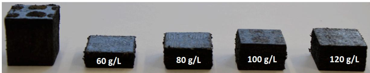
**Figure 1.** Results of dynamic compression test of EPS foam at high temperature  $\approx 50^{\circ}\text{C}$ .
