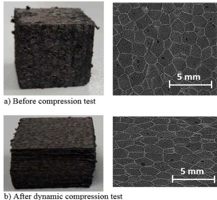
**Figure 4.** CT-scan images of EPS foam before and after dynamic compression test (Foam density = 60 g/L, low temperature ( $\approx -20^{\circ}\text{C}$ )).
