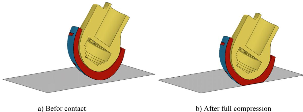
**Figure 7.** Predictions of the helmet impacting the crown site on the road.
