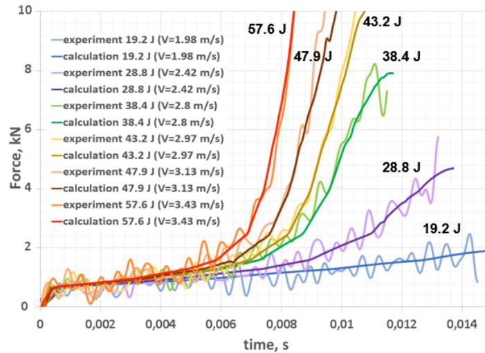
**Figure 5.** Comparison between the experimental and simulation results of the dynamic compression test (Foam density = 80 g/L, low temperature ( $\approx -20^{\circ}\text{C}$ )).
