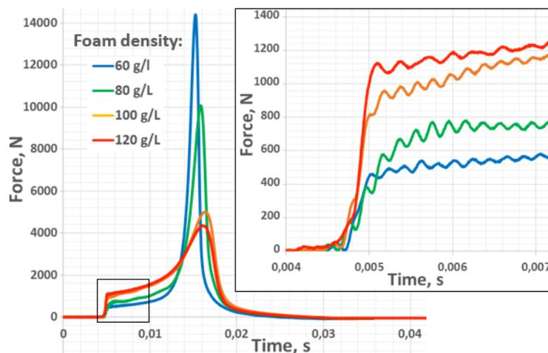
**Figure 2.** Dynamic compression test results (room temperature ( $\approx 18^\circ\text{C}$ )).
