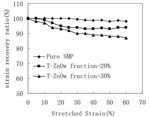
Fig.2. The strain recovery ratio ver stretch strain for different T-ZnO<sub>w</sub> fraction
