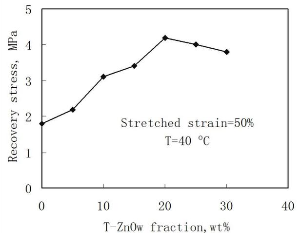
Fig.3. The recovery stress ver T-ZnO<sub>w</sub> fraction
