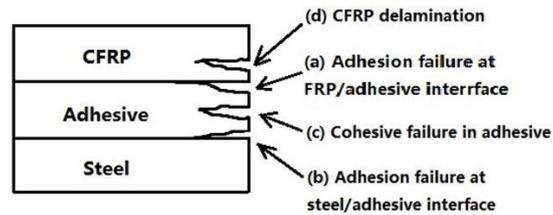
**Figure 1.** Possible failure modes of FRP-to-steel bonded joints.
