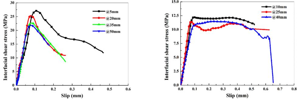
**Figure 6.** Bond-slip relationship curve for T1 and Tc in CFRP delamination failure.
