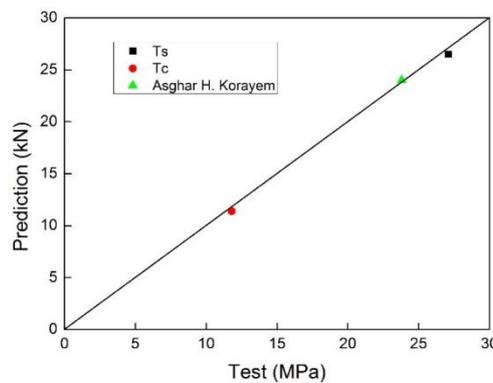
**Figure 7.** Comparison between the test and predicted maximum shear stress
