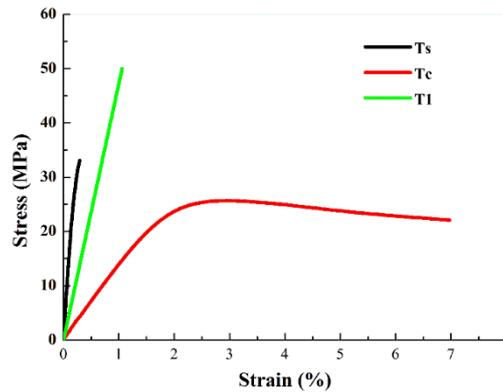
Figure 2. Tensile stress-strain curves of three adhesives.
