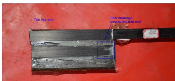
**Figure 4.** CFRP delamination failure mode.
